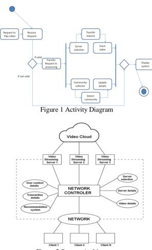
Figure 2 System Architecture
